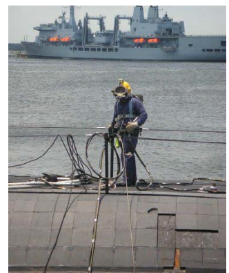
(Below) Logan diver Chris Davis performs towed sonar array repairs to a Royal Navy Submarine in Jacksonville, Florida.
